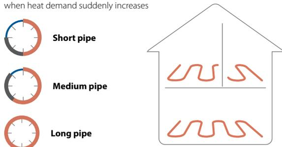
**Small rooms** with short pipes experience limited pressure losses. Therefore, the short pipe will "steal" most of the energy / water at the expense of the long pipes and will be heated quickly.
